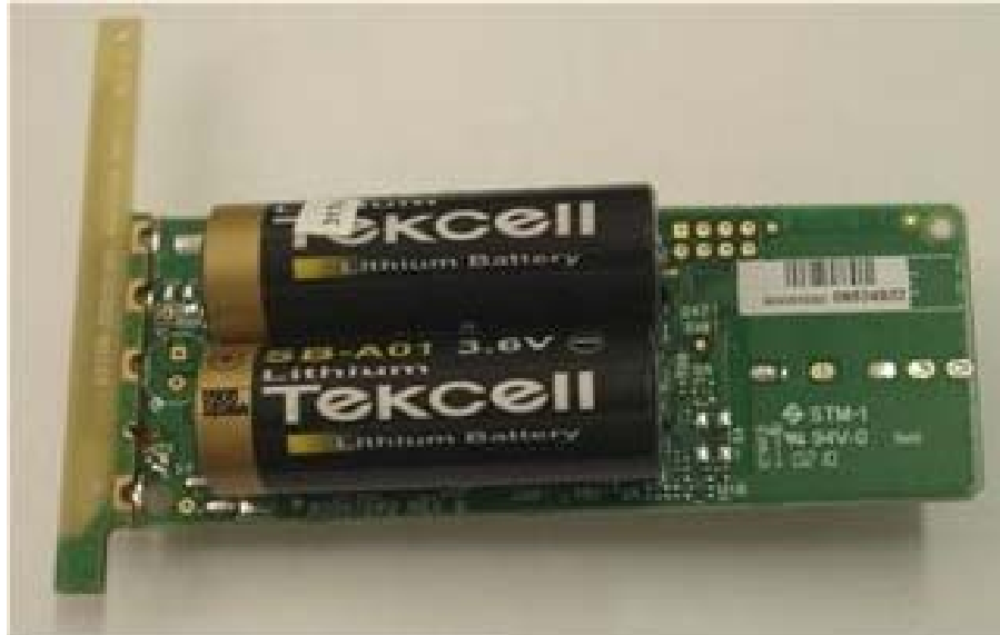
Photograph No.4 Booster 2 PCB with batteries
