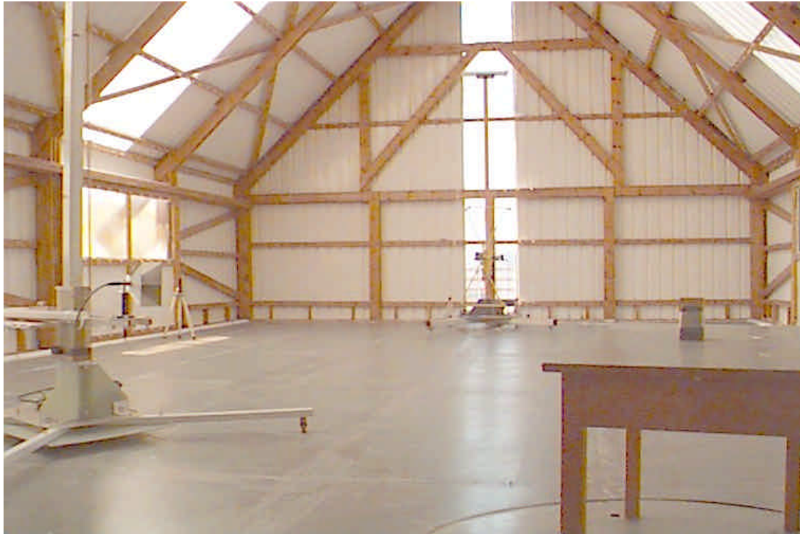
Setup for radiated measurements with double ridge guide antenna
