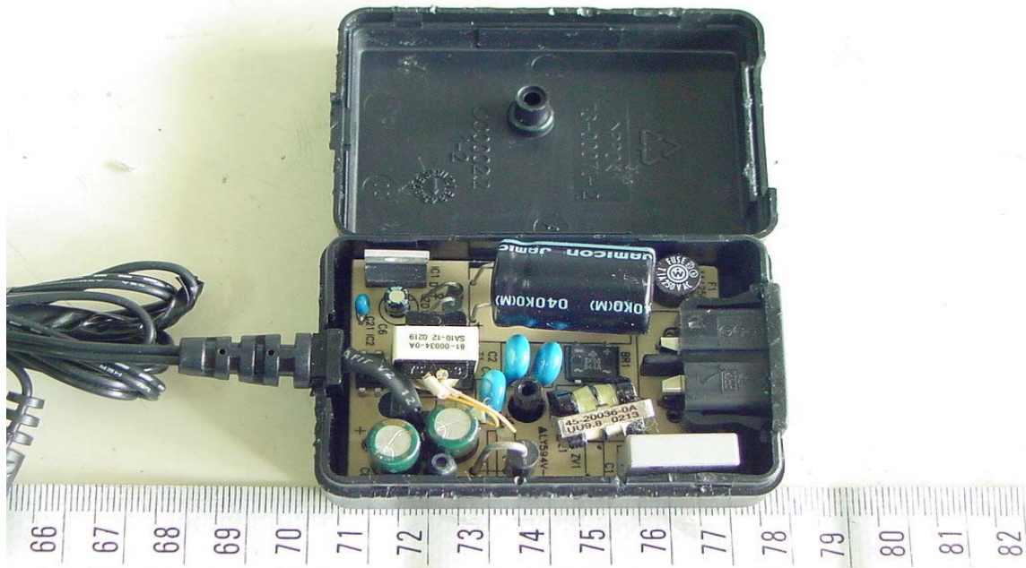
Component View of Adapter's PCB
