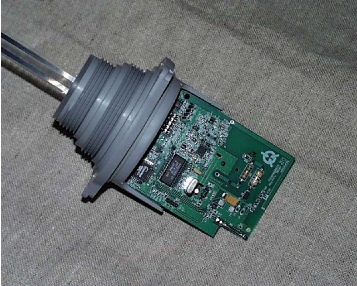
Figure 2: Photograph of circuit board assembled on base (1)
