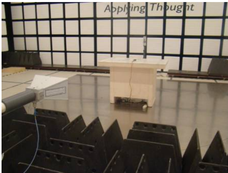
Figure 3: Test setup for Radiated Emission (Vertical) – 1GHz to 18GHz
