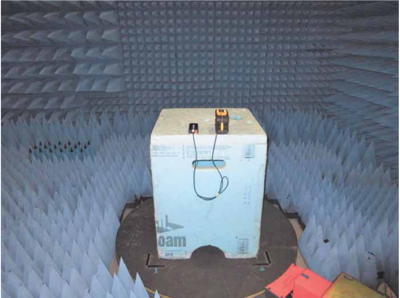
Radiated Above 1 GHz - USB Battery Bank Powered - Back
