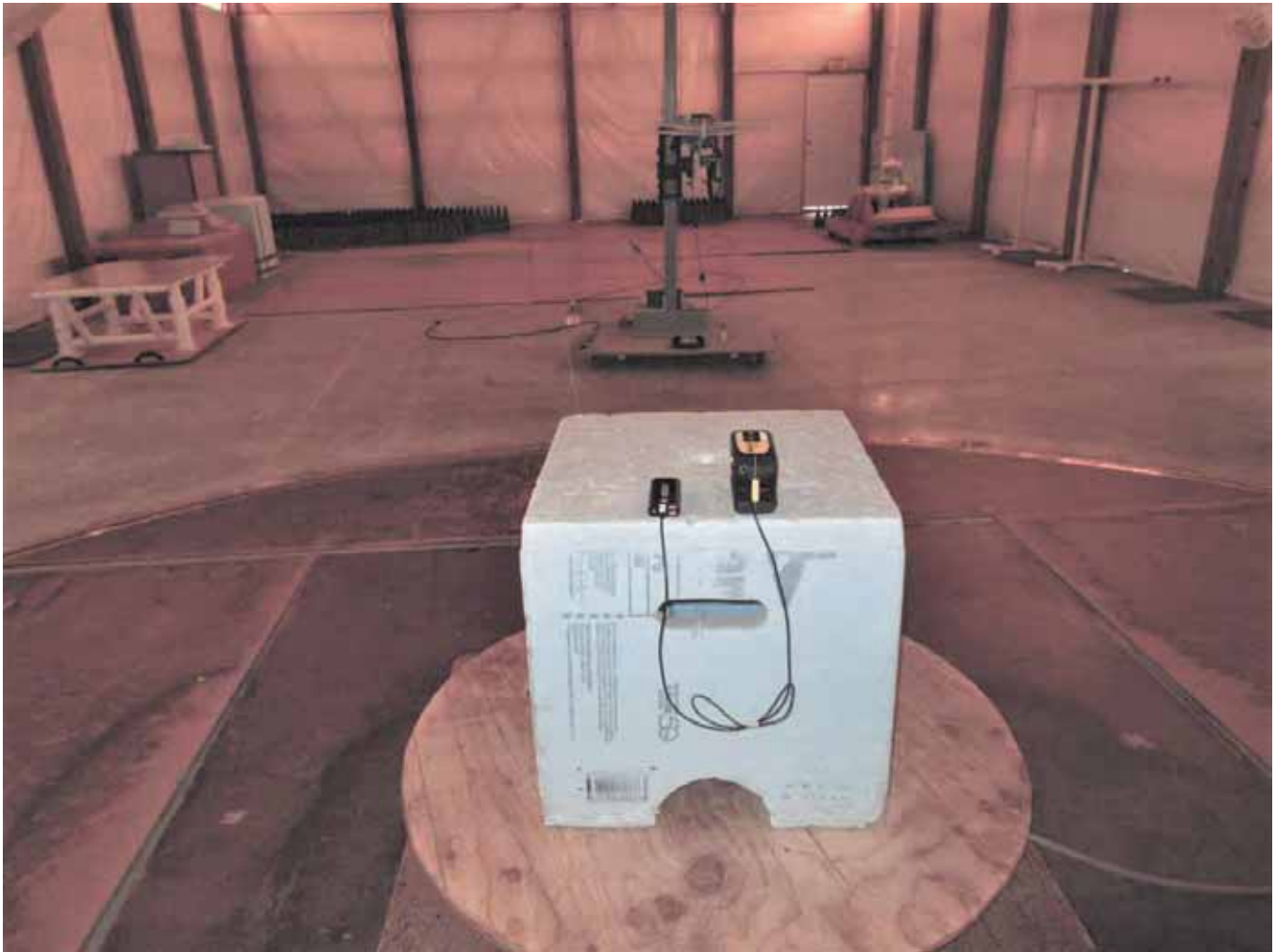
Radiated Below 1 GHz - USB Battery Bank Powered - Back
