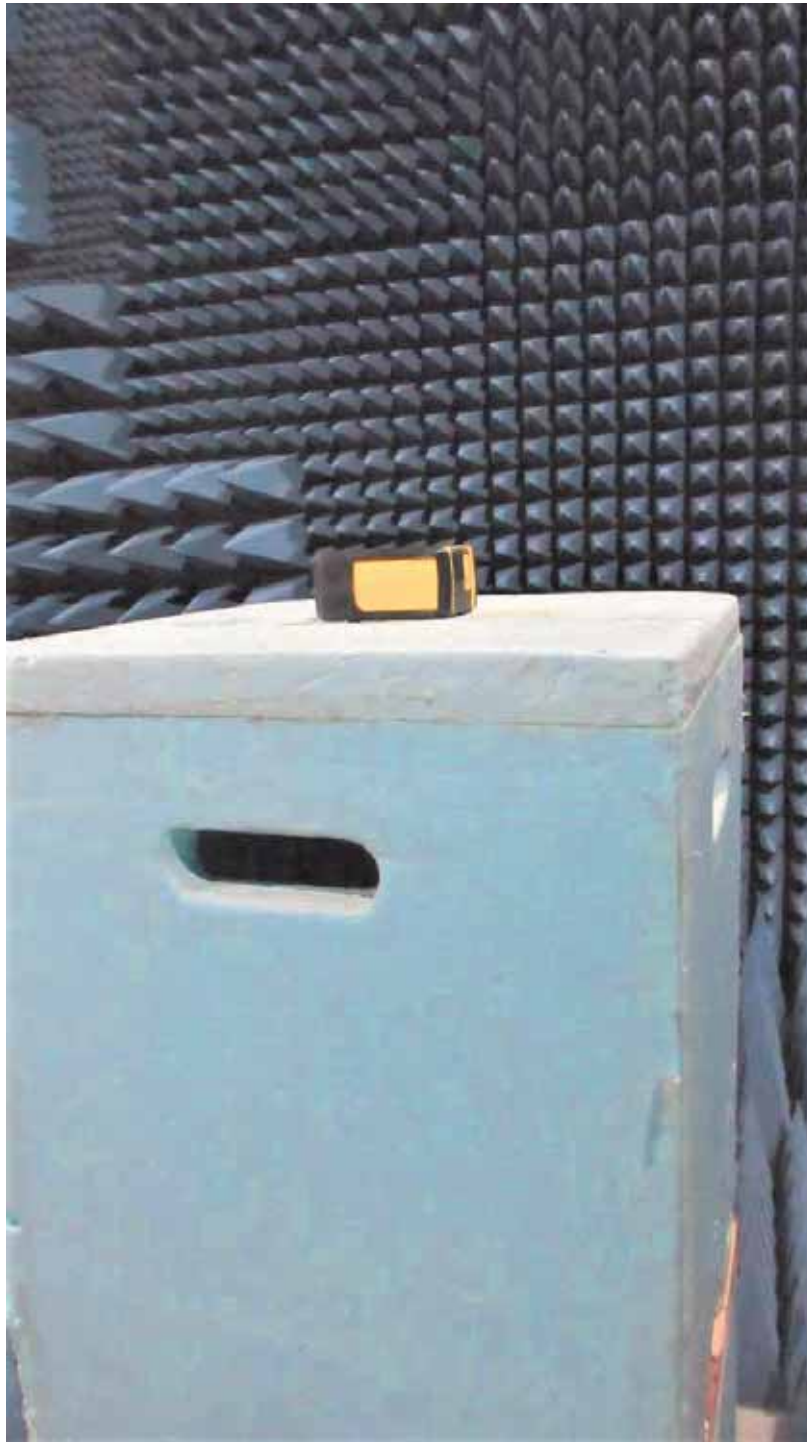
Radiated Above 1 GHz - Battery Powered
