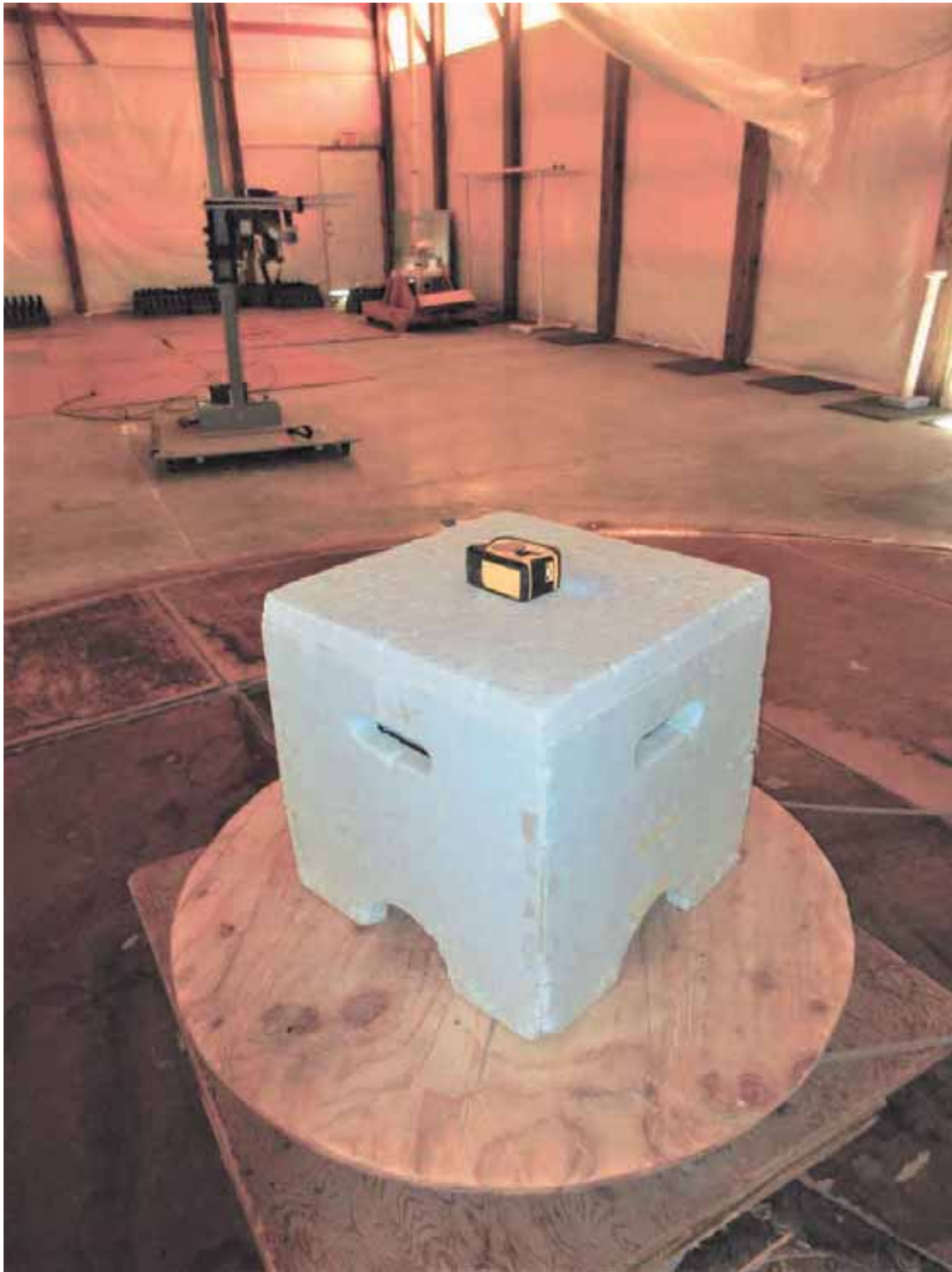
Radiated Below 1 GHz - Battery Powered
