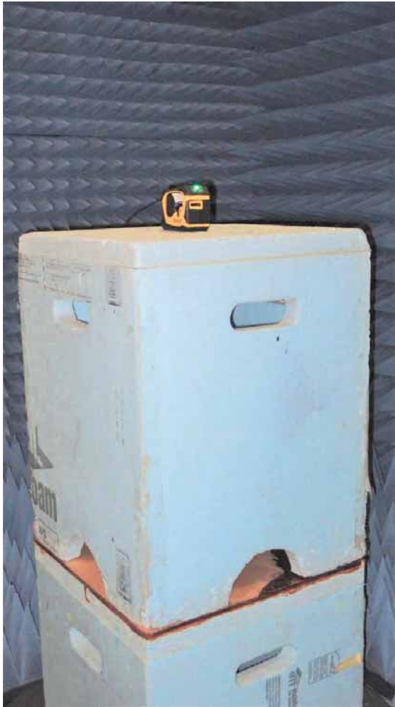
Radiated Above 1 GHz - USB Powered - Front
