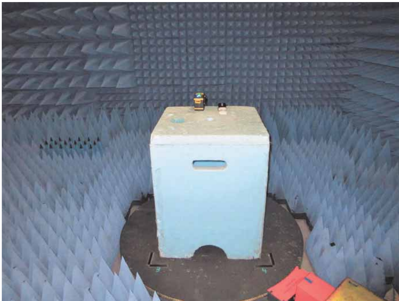
Radiated Above 1 GHz - USB Battery Bank Powered - Front
