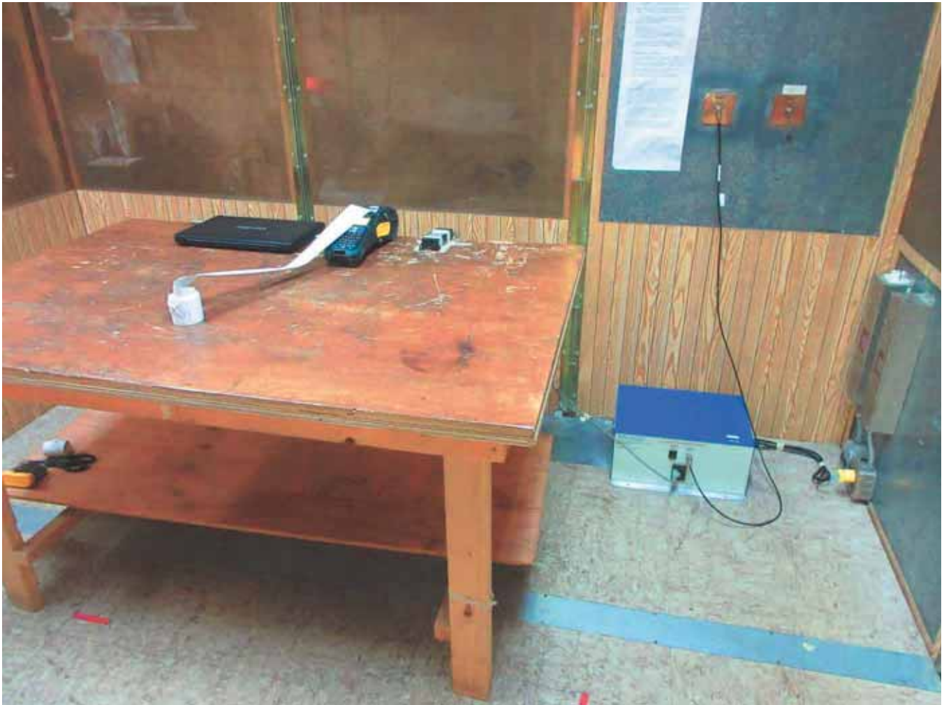
AC Line Conducted Emissions - Front
