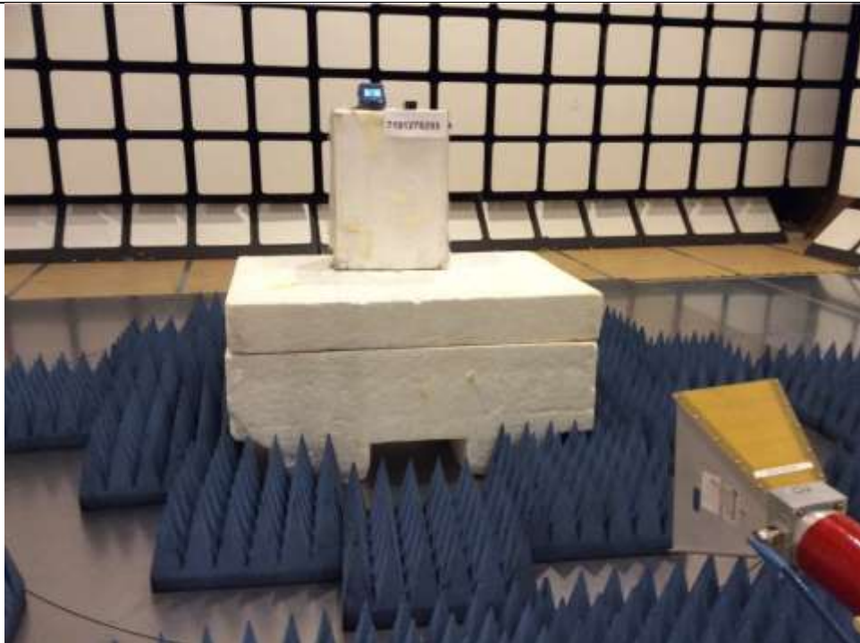
Radiated Emissions (Spurious Emissions Inclusive Restricted Bands Requirement) Test Setup (Front View)
