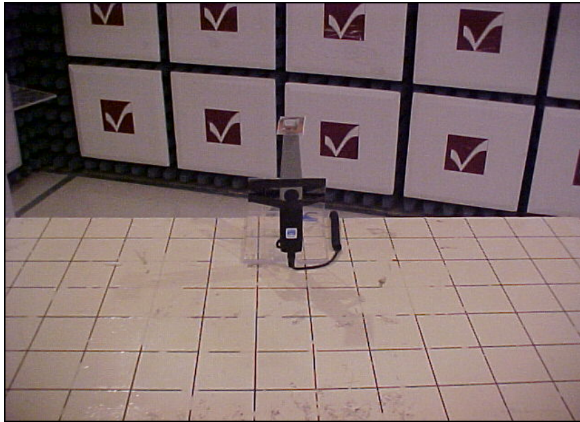
Photo(s) of Setup for Radiated Emissions Test Brady Worldwide FCC ID #: NUC-BEPM13
