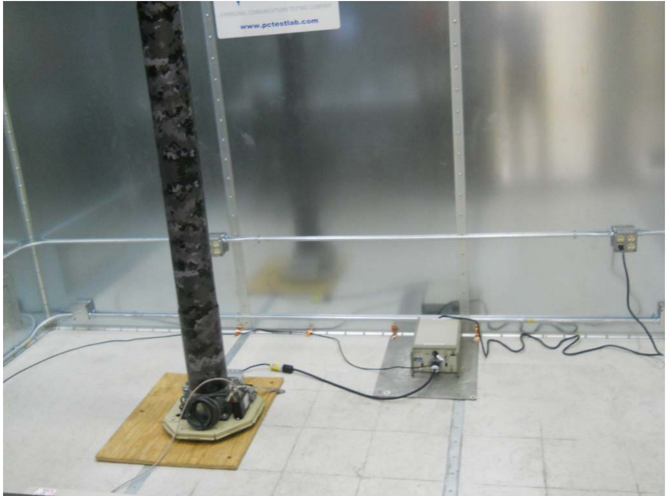
Figure 1. AC Line Conducted Test Setup
