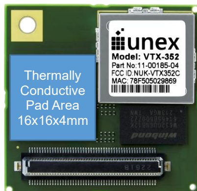
Figure 7: Recommended Thermally Conductive Pad Area
