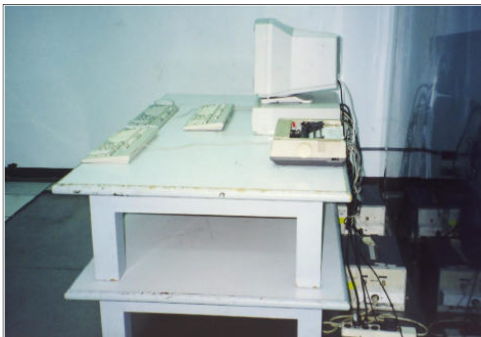
Conducted Emission Setup Photos (Worst Emission Position)
