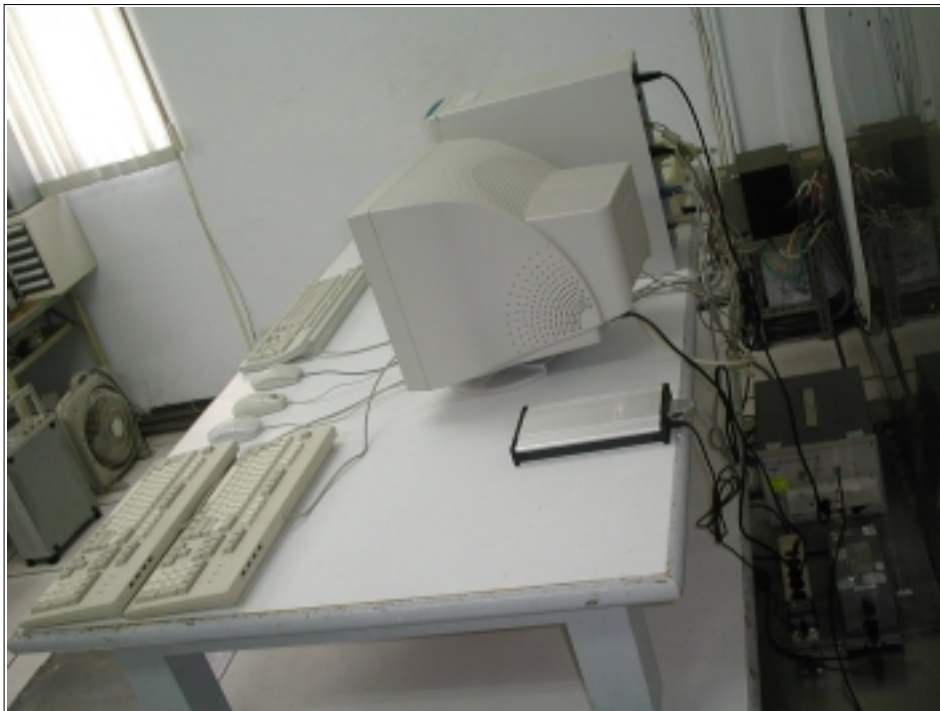
Conducted Emission Setup Photos (Worst Emission Position)
