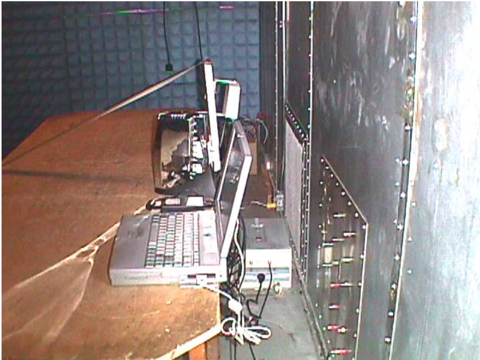
Test setup for AC Power-line Conducted Emissions in a Shielded Chamber (Side View)
