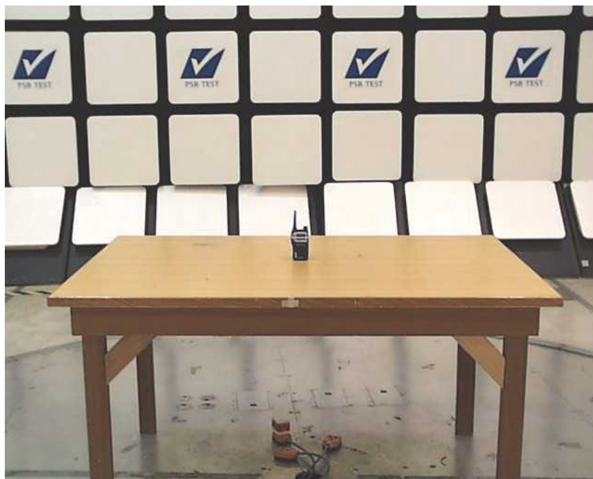
Effective Radiated Power Test Setup General View
