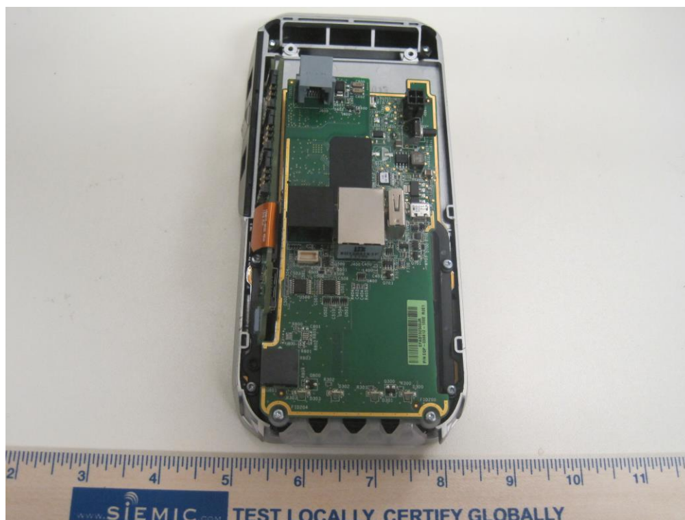
EUT Main Board
