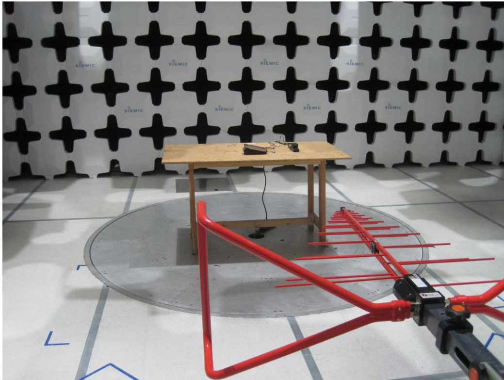
Radiated Emission (<1GHz) – Front View
