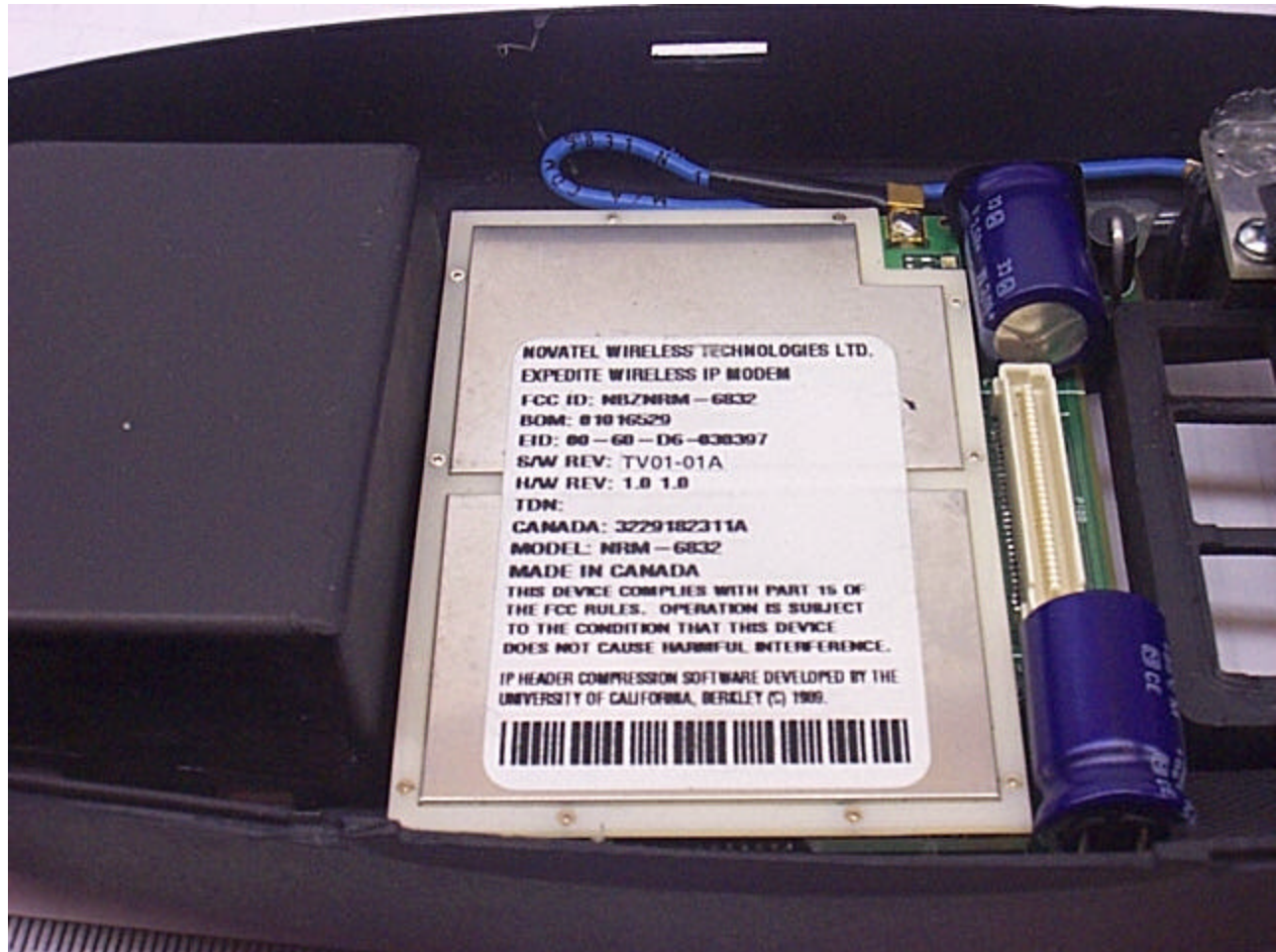
Hypercom Point of Sale Device SmartICE with a Novatel NRM-6832 transmitter CDPD: Back Open, detail, transmitter
