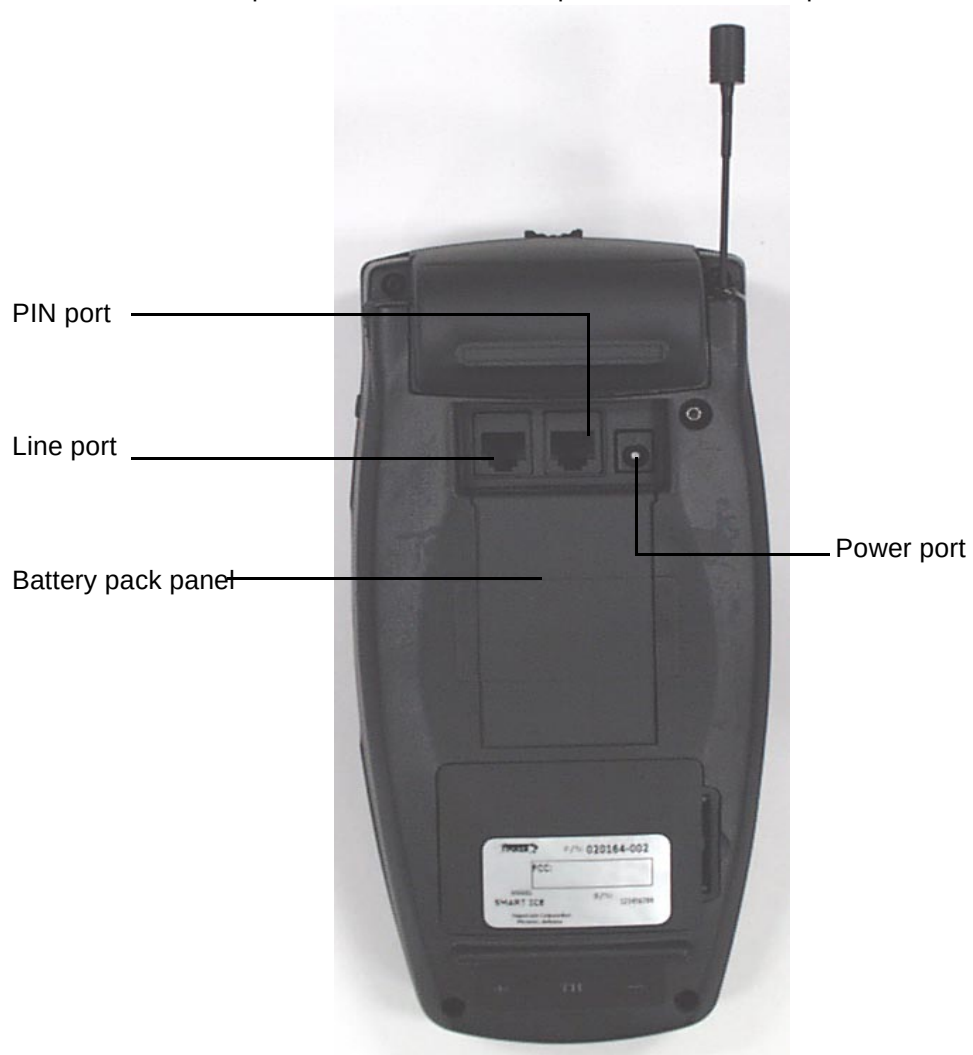
Figure 2-1. SmartICE under panel connectors
