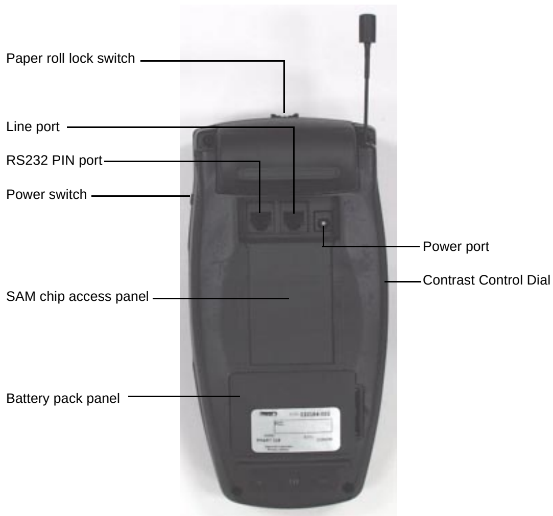
Figure 2-1. ICE 4000 under panel connectors
