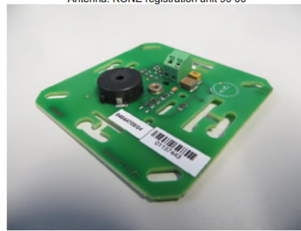
Antenna: KONE registration unit 90 00
