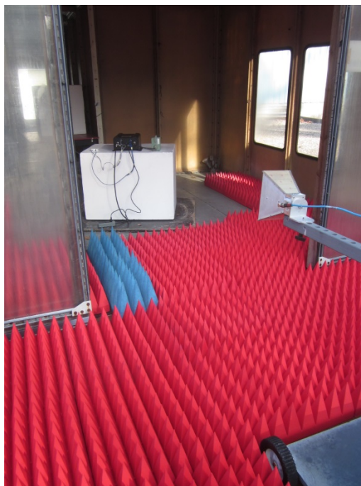
Spurious Emissions, Double Ridge Guide, 1-10 GHz, Horizontal Polarization
