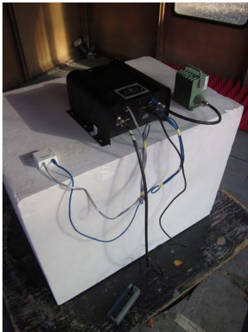
Spurious Emissions, Radiated, Test Setup
