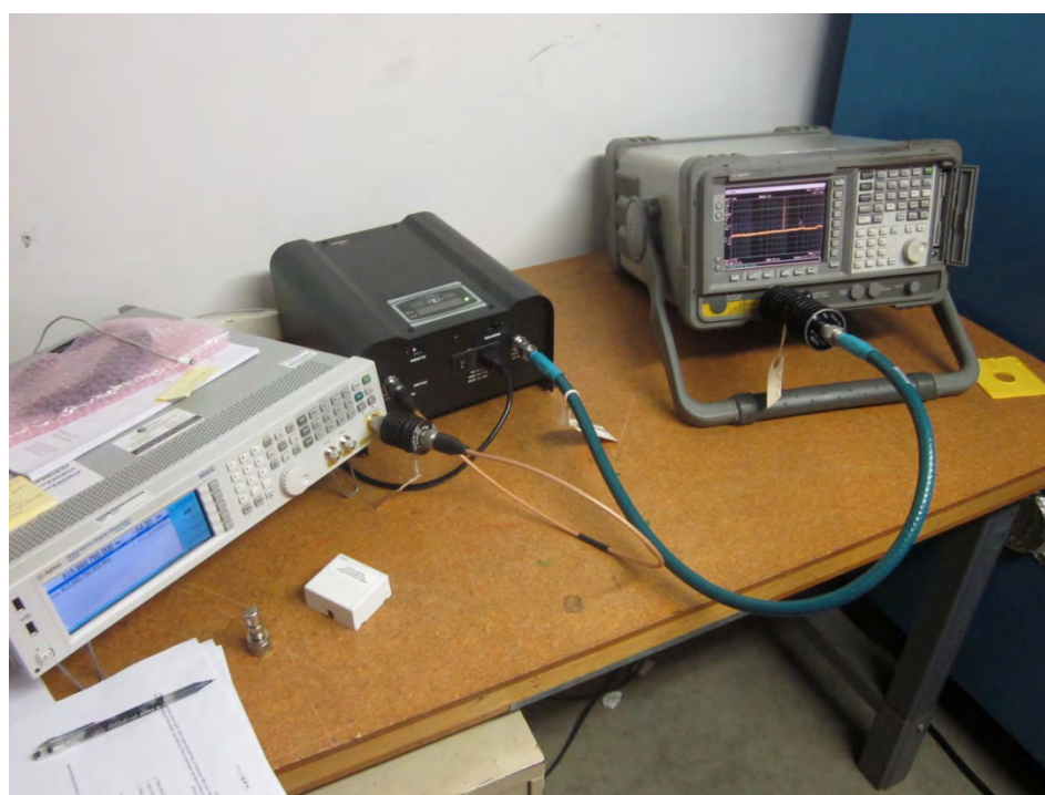
Spurious Emissions Conducted, Test Setup
