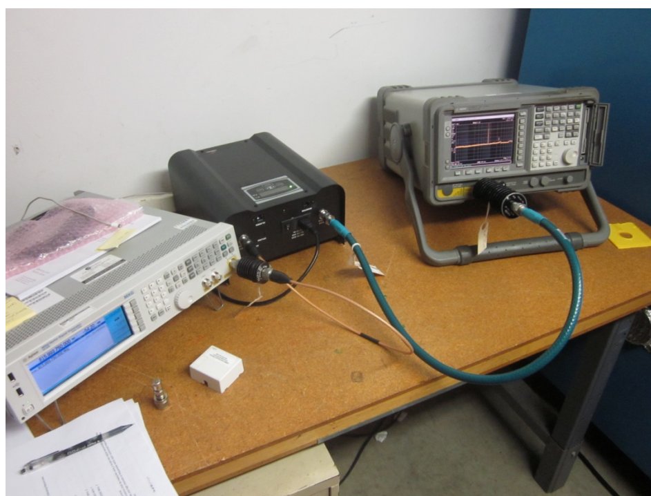
Spurious Emissions Conducted, Test Setup
