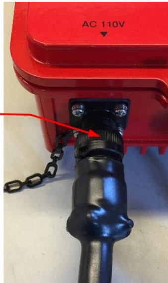
Figure 5-9: Power Cable Connected to Repeater
