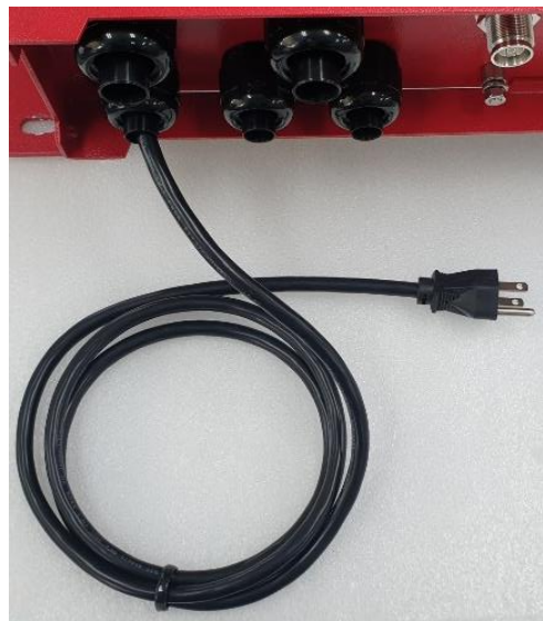
Figure 5-9: Power Cable Connected to Signal Booster
