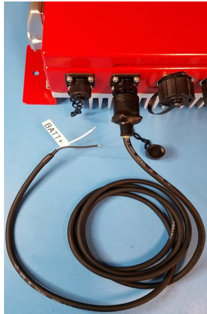
Figure 5-11: Battery Cable Connected to Signal Booster
