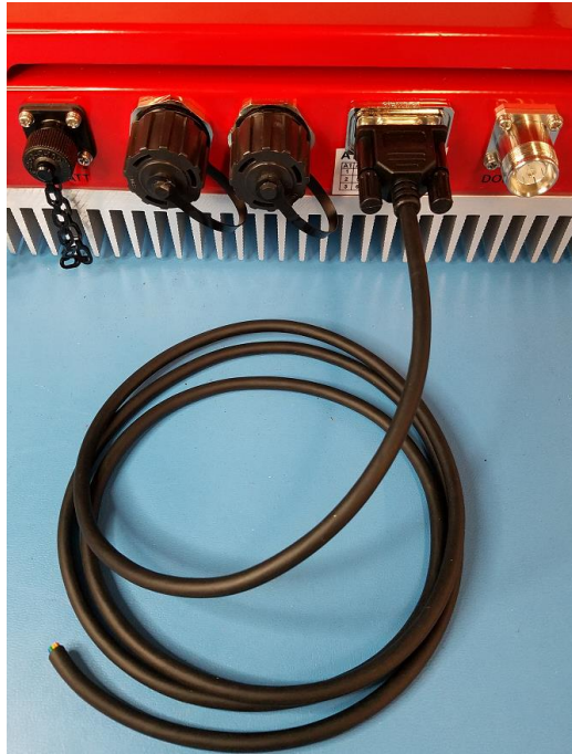
Figure 5-6: Alarm Relay Cable Connected to Signal Booster
