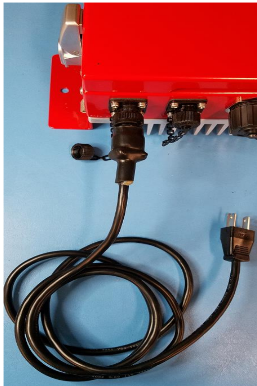
Figure 5-10: Power Cable Connected to Signal Booster
