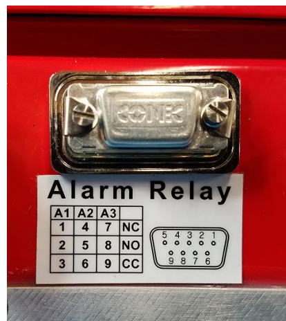
Figure 5-5: Alarm Relay 9 Position D-Sub Connector
