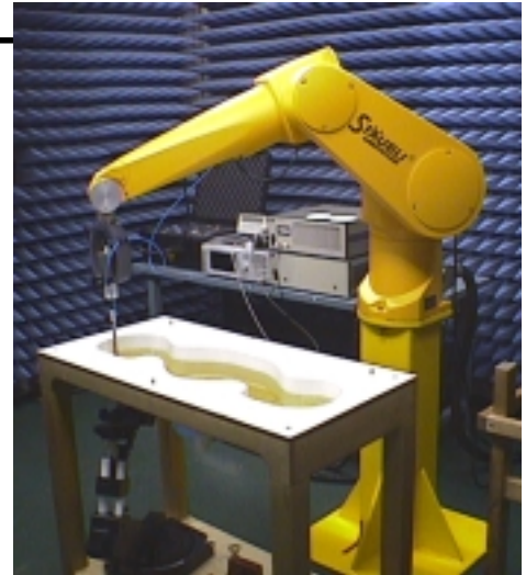
Fig1: The robot controlled probe during SAR measurement.
