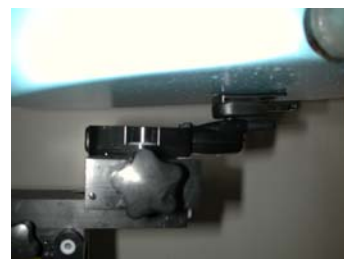
Figure 22. Body SAR Test Setup
