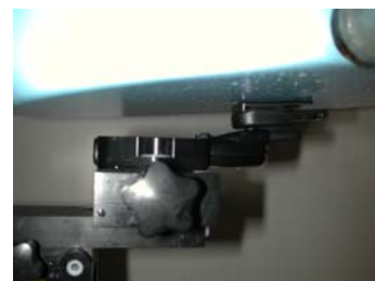
Figure 21. Body SAR Test Setup
