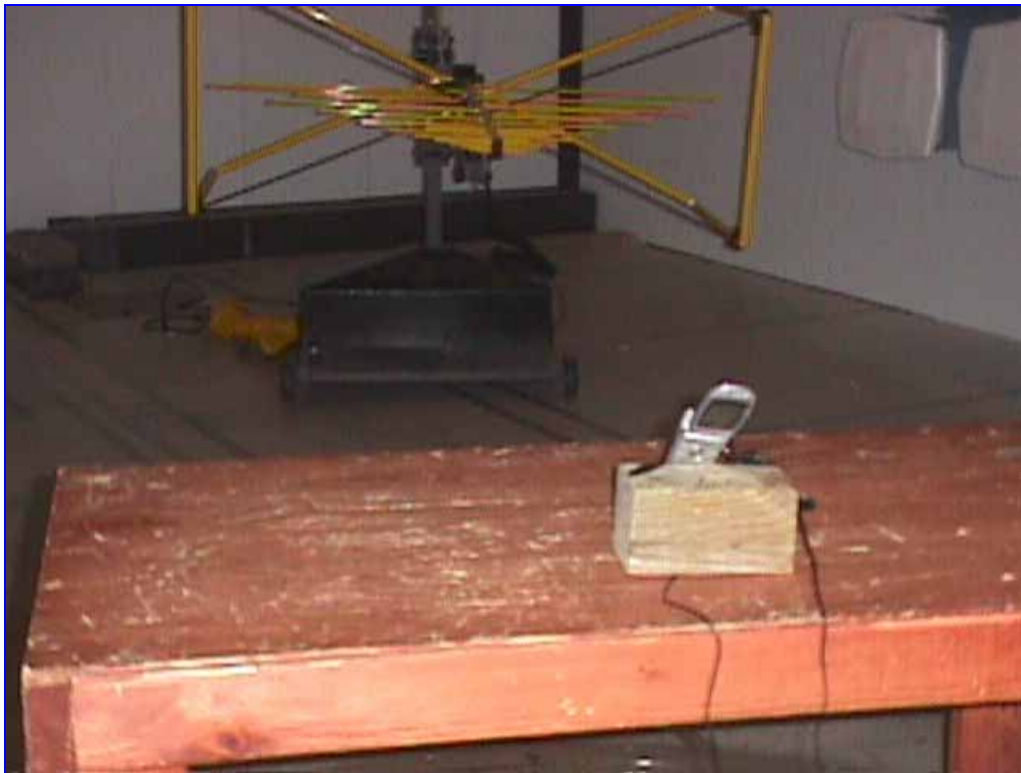
Photograph 2. Intentional Radiated Emission Limits, Test Setup
