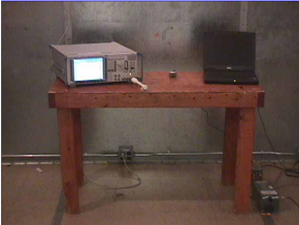
Photograph 1. Conducted Limits, Test Setup
