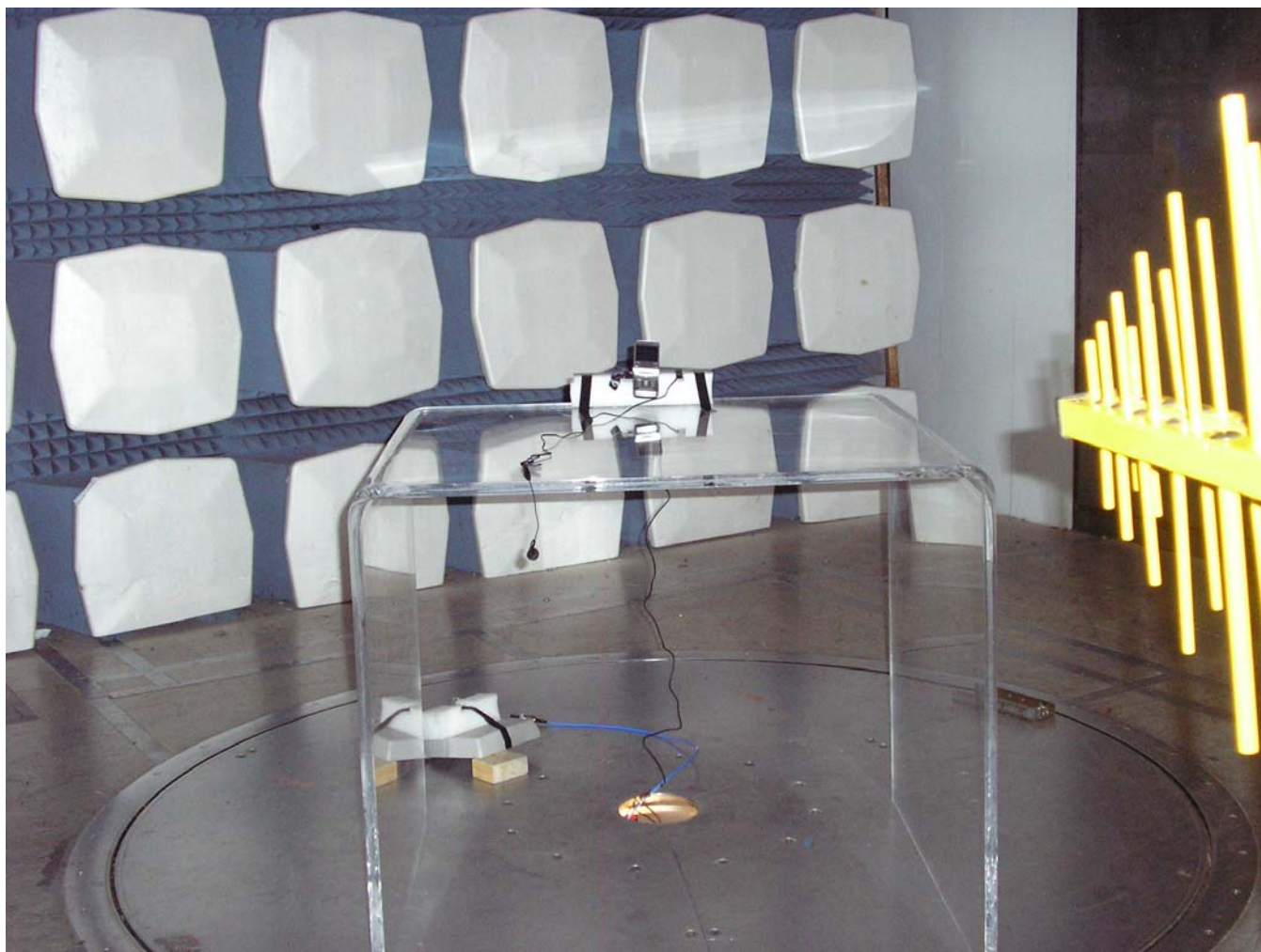
Photograph 5 Radiated emissions measurement Setup
