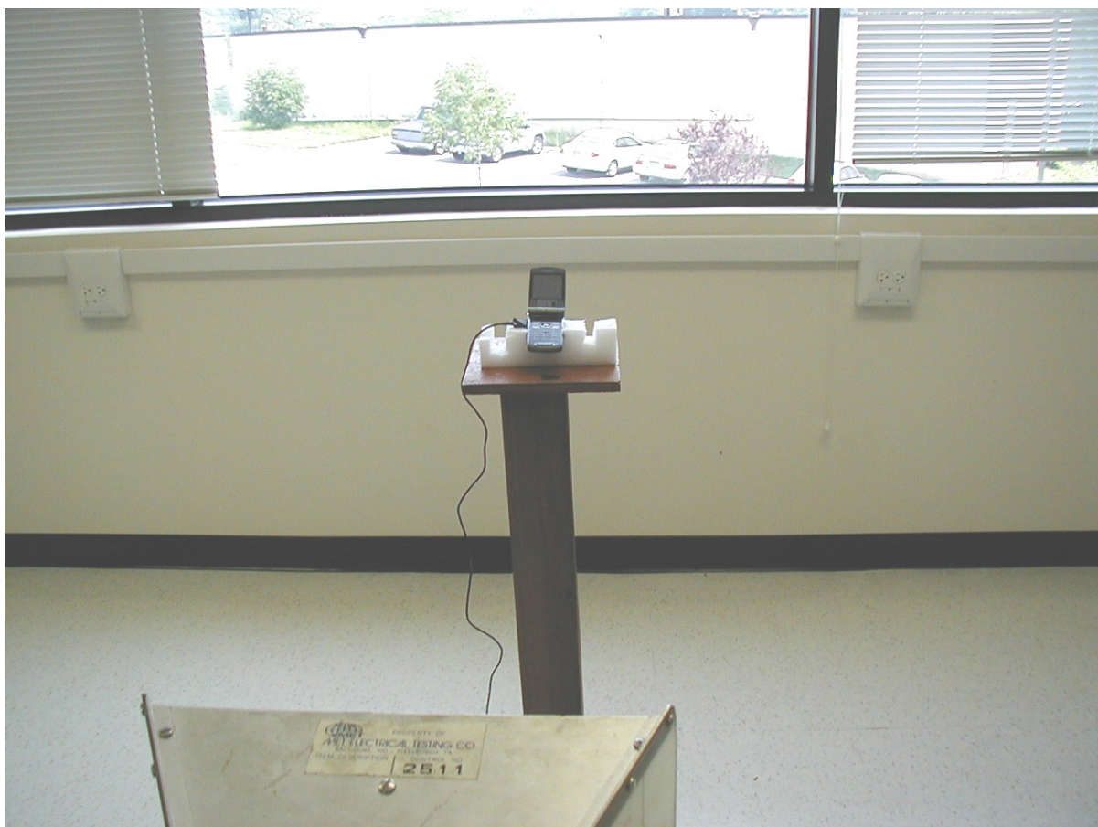
Photograph 6 Radiated emissions measurement Setup
