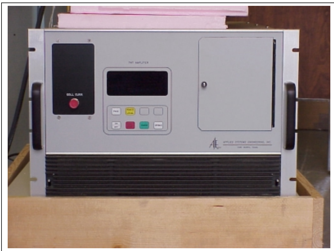
Figure 1 – Traveling Wave Tube Amplifier Assembly (Front View)
