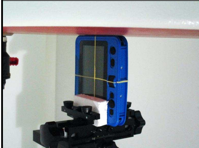
Left Side of EUT with 0 cm Gap
