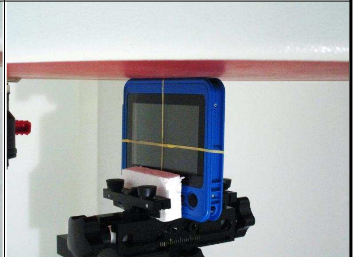
Bottom Side of EUT with 0 cm Gap
