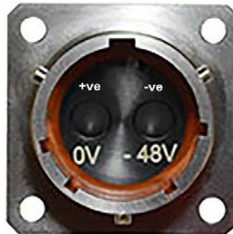
Figure 3-7 –48 V DC 2-pin Rosenberger bulkhead jack
