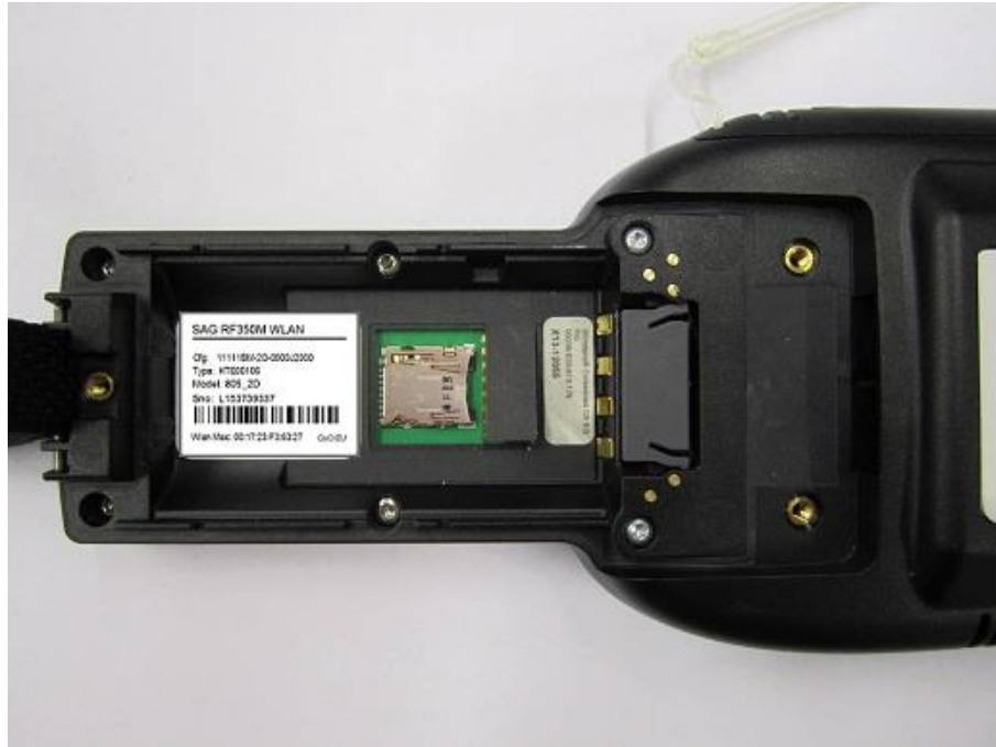
Picture 6. Simatic RF350M inside label location.
