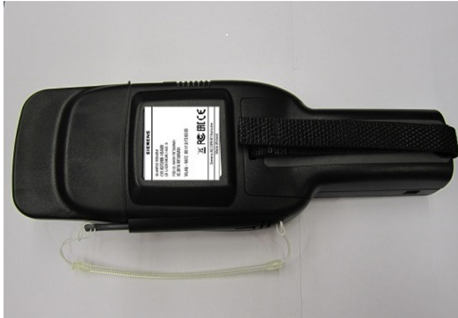
Picture 5. Simatic RF350M outside label location.
