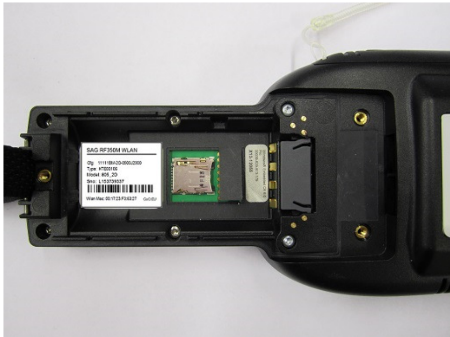
Picture 6. Simatic RF350M inside label location.
