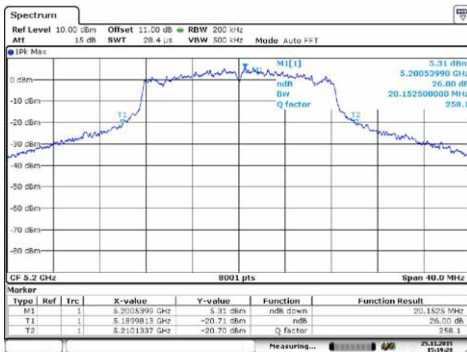
Screenshot: Occupied 26 dB bandwidth Measurement, channel 36
