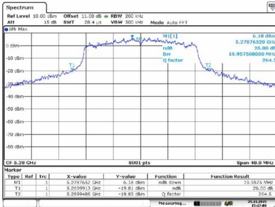
Screenshot: Occupied 26 dB bandwidth Measurement, channel 56
