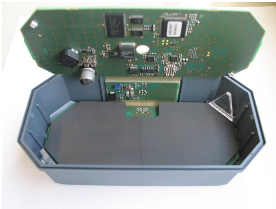
Fig. 4: PCB fixed in housing with ferrite
