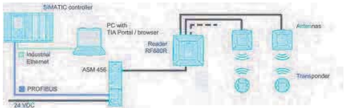
Figure 8-3 Configuration graphic with SIMATIC RF680R (or RF685R, RF610R, RF615R) and PROFIBUS connection
