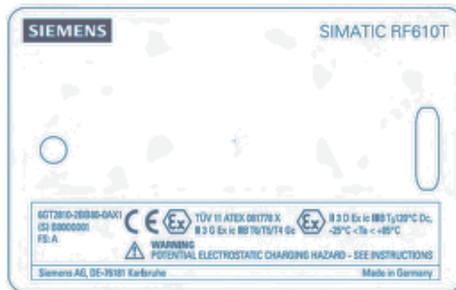
Figure 7-15 Schematic representation of the SIMATIC RF610T ATEX transponder
