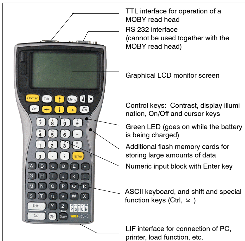
Figure 7-5 Hardware of the MOBY-I hand-held terminal STG
