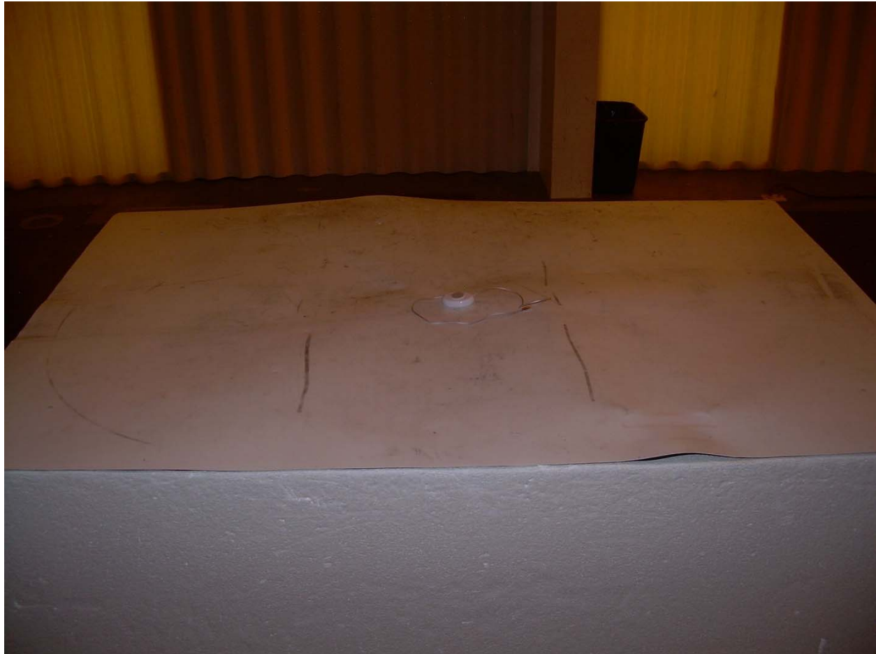
Photograph 4 – Front View Radiated Disturbance – Horizontal Configuration
