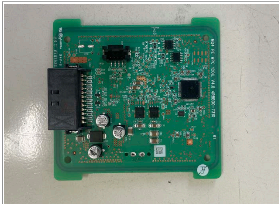
Bottom view of Main PCB
