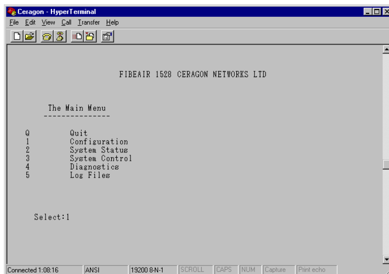
Figure 4-2 FibeAir 1500/1528 Terminal - Main Menu
