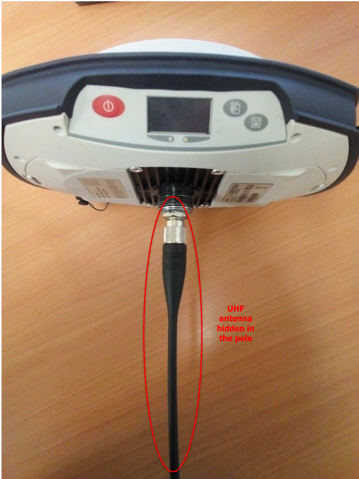
UHF antenna without the pole
