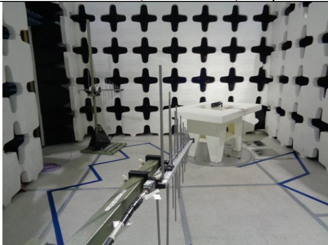
Class B Horn (1000-18000MHz) Setup
