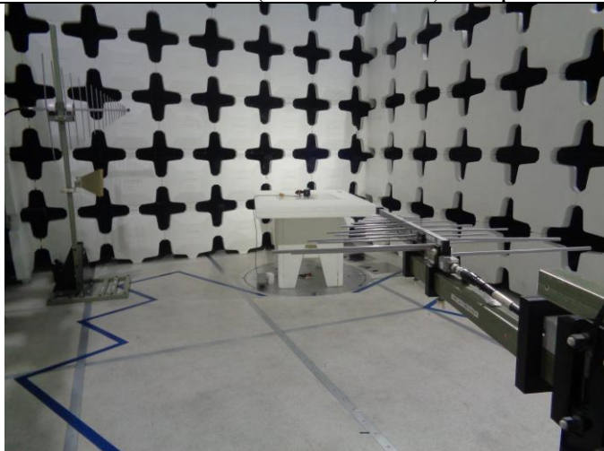
Class B Horn (1000-18000MHz) Setup
