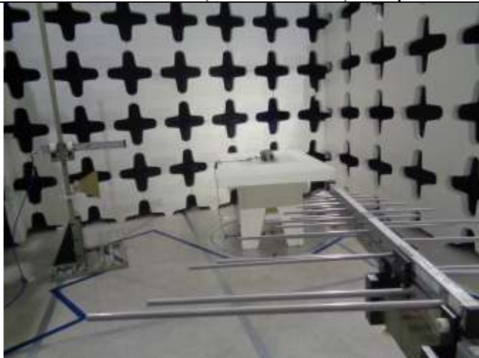
Class B Horn (1000-18000MHz) Setup
