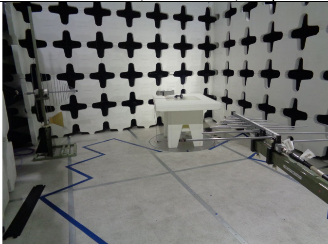
Class B Horn (1000-18000MHz) Setup
