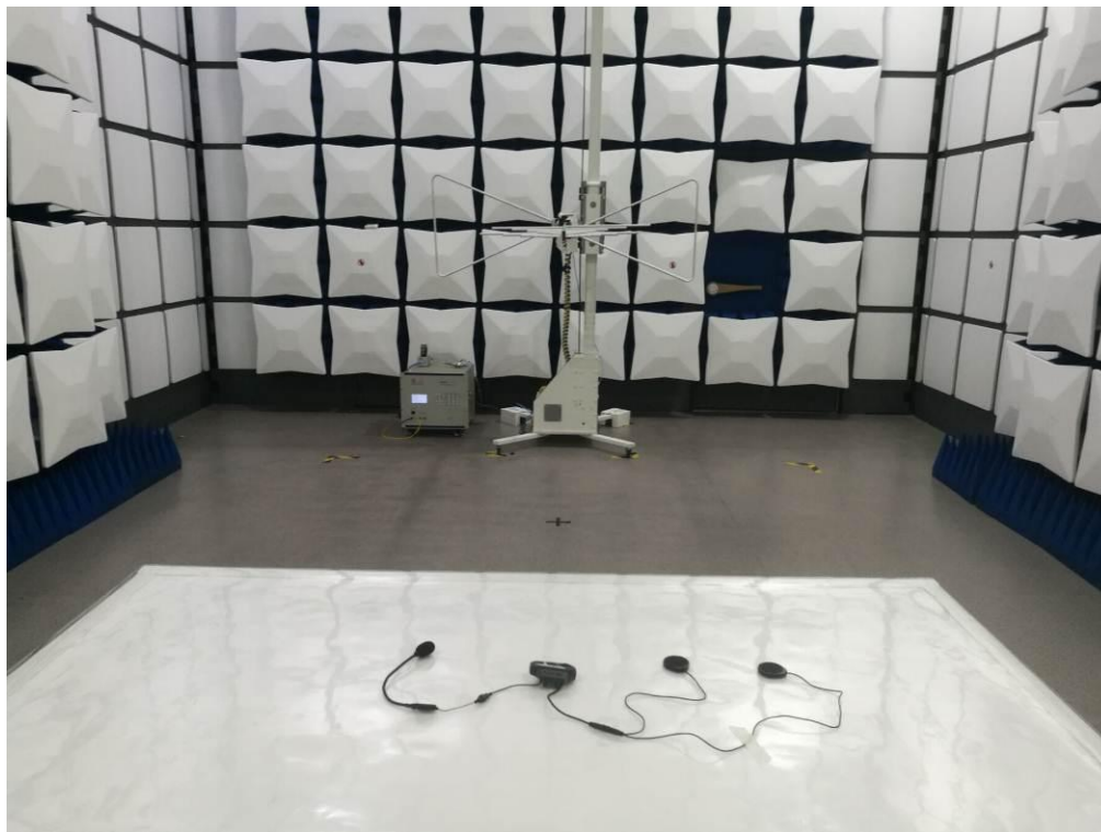
FCC RADIATED EMISSION TEST SETUP
