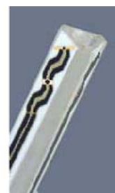
Figure 3.2 Probe Thick-Film Technique
